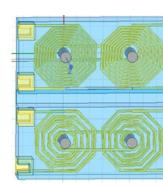
Besides the sensor coils, we are exploring advances in other multi-material Additively Manufactured Electronics (AME) assemblies to replace the wiring and machined structure and to integrate the coils and electronics. This is traditionally a very expensive machined part with grooves and channels to mount the coils and hand-route tiny wires to the sensor electronics. We are assessing 3D-printed ceramic parts for the sensor's structure and printed copper traces to replace the wires.
