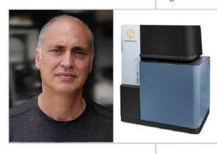
Avi Cohen, executive vice president at Nanofabrica, says that the company's Tera 250 DLP 3D printing platform has an optical system sharpness that delivers a pixel size of 1.9 microns and a layer thickness of 1 micron. The machine also has a rigid granite table and specialized servo elements and controls that enable precise movements for accurate, high-resolution micro parts.
